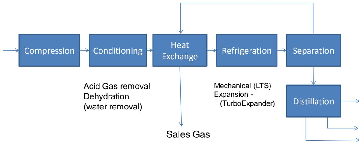
Cooling of the gas in the original plant is done by propane refrigeration in a conventional Low Temperature Separation (LTS) plant with a capacity of 15 MM SCFD. Dehydration is accomplished at the same time as hydrocarbon recovery, and freeze up is prevented by injecting glycol.
