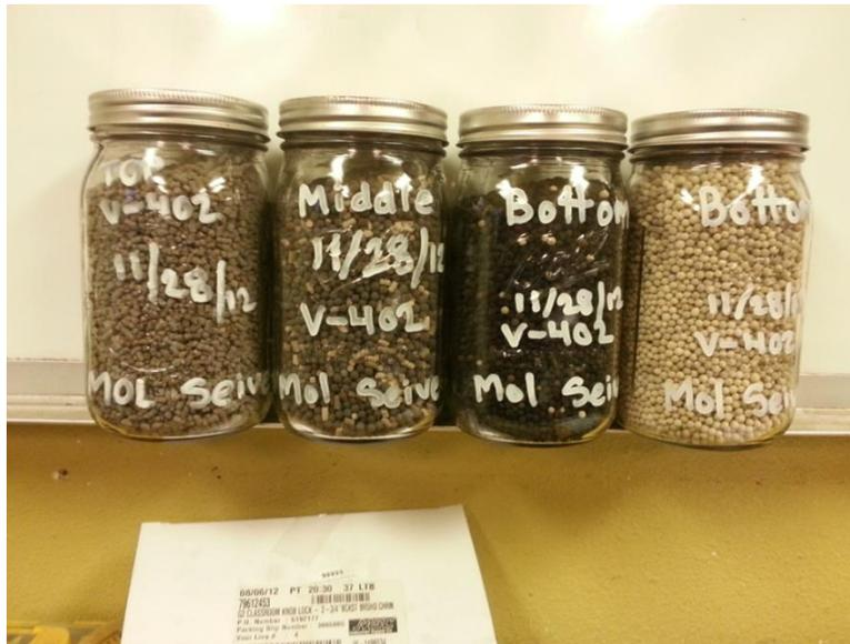
While the coking is self-evident, it should be noted that the mol sieve in both vessels V-402 and V-403 was easily removed, and flowed freely from the bottom of the vessels. There was no indication of clumping or damage due to the presence of free water. Also, there is essentially no discoloration of the ceramic balls and rather severe discoloration of the mol sieve directly above the ceramic balls.
