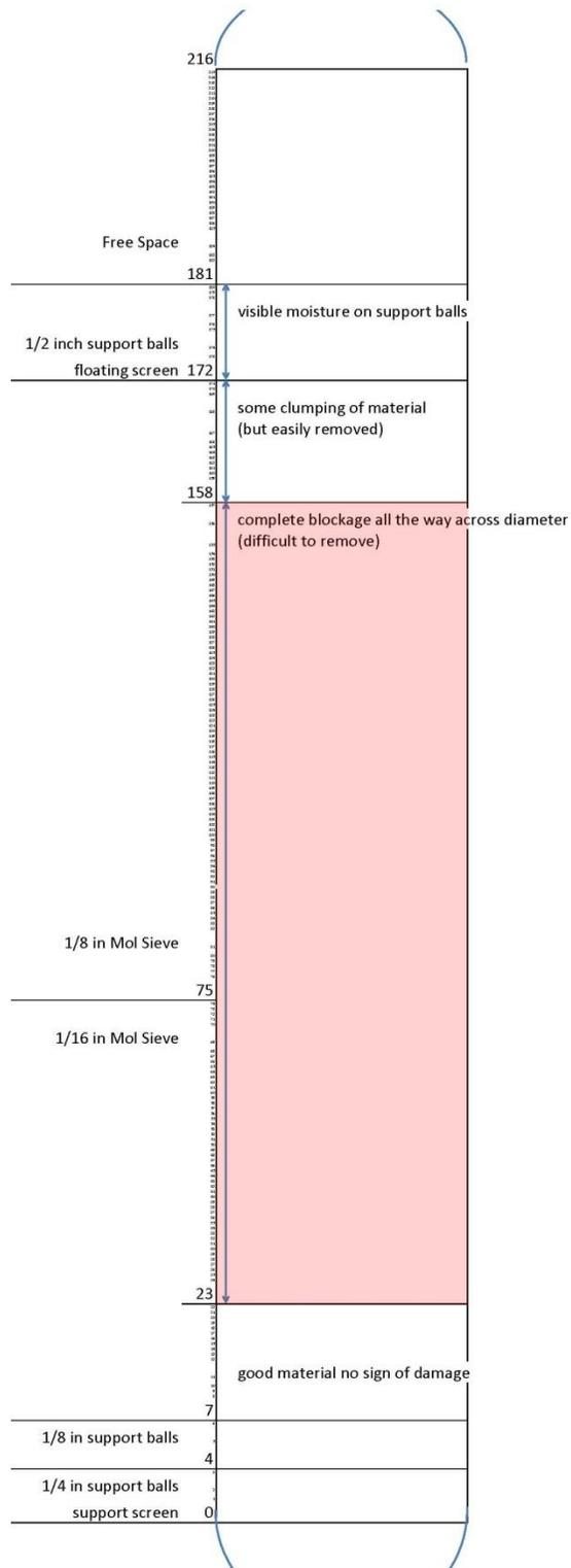
The most likely cause of free water is “refluxing” during the initial regeneration period where rising hot gas saturated with water from the mol sieve being regenerated encounters cold mol sieve material above it.
