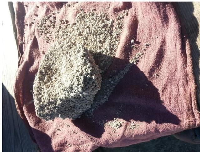
Opening the bottom hatch of the vessel to remove the mol sieve, good material without damage flowed freely from the vessel. However, only the material up to the 23 inch mark (from bottom seam) flowed freely from the vessel. At the 23 inch mark there was blockage across the entire diameter resulting in a block section from the 23 inch mark to the 158 inch mark (58 inch from top seam). The depth of the blocked section was therefore  $158 - 23 = 135$  inches.
