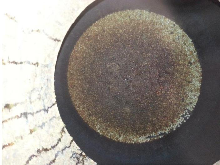
Below the floating screen clumps were observed in the mol sieve. However, the clumps were in sections and not uniform across the diameter. Also, the material was easily removed by vacuum.
